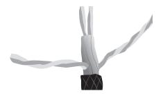
5 Thread the inner pairs (4/5, 3/6) through the wire tray and seat the wires in the proper slots as shown below. Then route the outer pairs on top of the wire tray and seat the wires as shown. Once the wires are pressed into the slots, trim the excess wires with a pair of flush-cutters.
