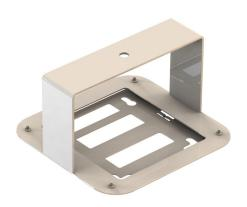
The AccelTex Solutions Universal All-Thread Drop Mount provides a unique solution to mount a Cisco, Aruba or other T-Bar mounted AP using All-Thread. The AP snaps into place by fitting the AP mounting feet into pre-defined keyholes in the mount or using the T-Bar mount supplied with the AP. This mount can be used to lower the height of the antenna and AP in a building with high ceilings or can even be placed above a suspended ceiling. All-Thread and fasteners not included.
