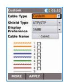
Use a list of wiremap templates for common Ethernet cable types as well as non-Ethernet cables, such as Profinet and ISDN.
