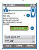
Press the Autotest button to display summary information and allow for detailed inspection of network parameters.
